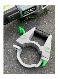
2. Before installing the handle onto the leaf blower, check to make sure that the orientation of both halves of the handle are correct.
