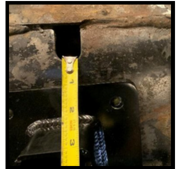
Bottom aligned with factory embossment.
