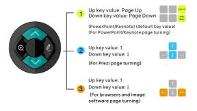
Note: It will vibrate once when switching, indicating that the switch is successful. The three key values can be switched cyclically.
