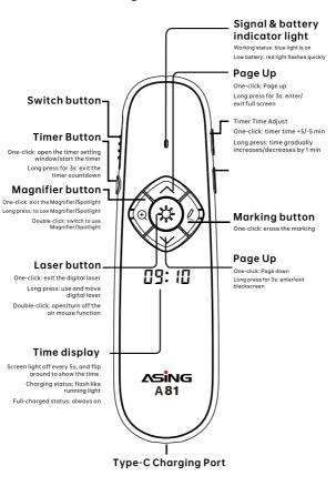
Using Tips: When long-pressing the Magnifier button, click the " \ " " \ " to shrink/expand the function areas. Same for Digital Laser.
