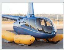
DART delivers superior safety for R44/R66 overwater operations with cylindrical floats made from lightweight urethane coated nylon.
