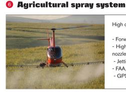
High capacity, gas or electric driven agricultural spray system for the R44/R66
