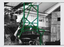
Eases hangar storage by allowing the rotor blades to be stowed in line with the helicopter fuselage. 2 people can fold and secure blades in 10 minutes. Can also be accomplished by a single person.
