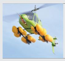
DART delivers superior safety for operators using their 505 in overwater application with Tri-bag floats made from lightweight urethane coated nylon.
