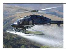
High capacity, electric driven agricultural spray system for the for Bell 407/206L.
