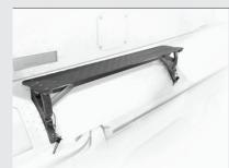
Provides a secure work platform for maintenance personnel to perform safe inspections on the main rotor and transmission.
