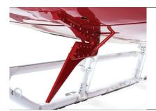
Prevent possible wire or cable strike on flight controls.
