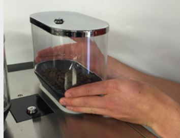
Refill hopper with product and place onto machine
