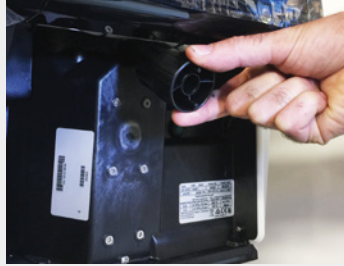
Turn pin left using the multi tool to release all hoppers
