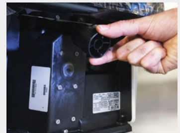
Turn the lock system to the right to re-lock hoppers
