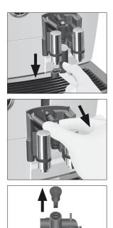
► Carefully pull the bottom part of the milk system down and off.
