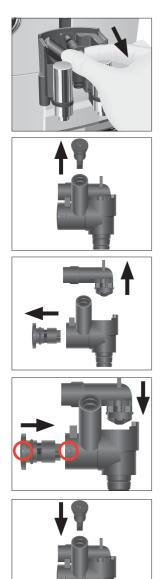
► Remove the milk system from the dual spout.
