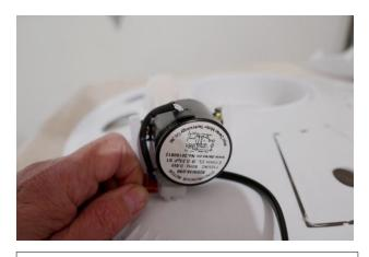
Tuck the wire and connector under the motor as much as possible. Leave a little excess cord under the motor so that it may be bent and exit easily through the notch in the cover.
