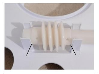
The gear may be slid slightly to the right or left to properly align it between the mounting posts. A very small gap should be visible between each end of the raised portion of the gear and the mounting posts. (areas pointed to by black lines above.)
