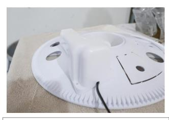
Place the cover over the motor and gear allowing the cord to exit through the notch in the bottom of the cover as shown. There's a single screw in the cover for screwing it down onto the reservoir lid.
