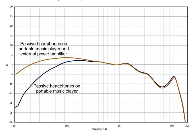
In this example we see a typical hi-end balanced armature headphone with a 25 ohm impedance.
