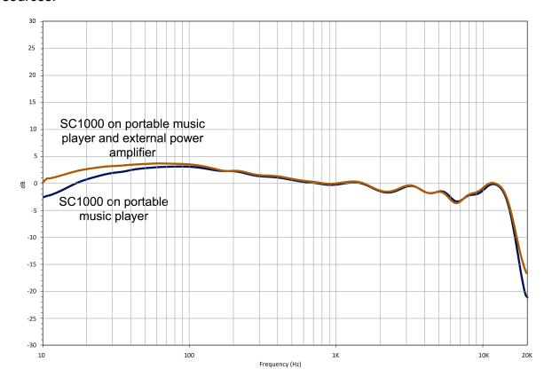
The power amplifier in the SC1000 has a very low output impedance and it is virtually the same at all frequencies. The small, 2 dB loss at 20Hz is a result of the portable player trying to drive the 150 ohm input impedance of the SC1000's pre-amplifier.
