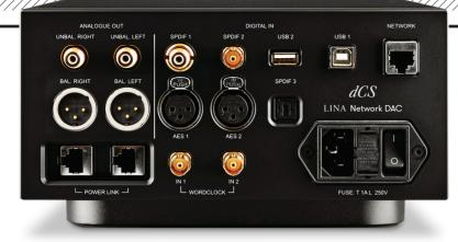
**ABOVE:** The Lina DAC 2.0 includes LAN, USB-B and USB-A (DSD128/384kHz), dual-AES (384kHz), 2x coaxial (192kHz) and optical (96kHz) inputs. Analogue outs on XLRs and RCAs are joined by Word Clock inputs for connection to the Lina Master Clock
