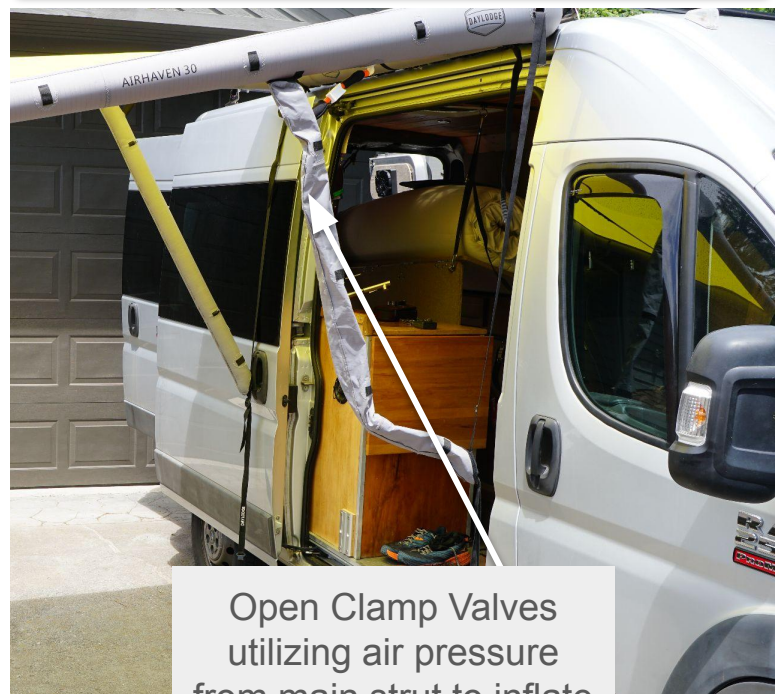
4- Pressurize struts to bring canopy into position
