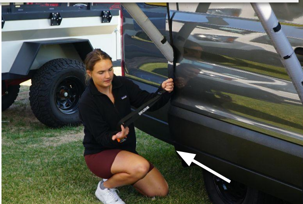
5- Secure and tension flat hooks to bottom of vehicle
