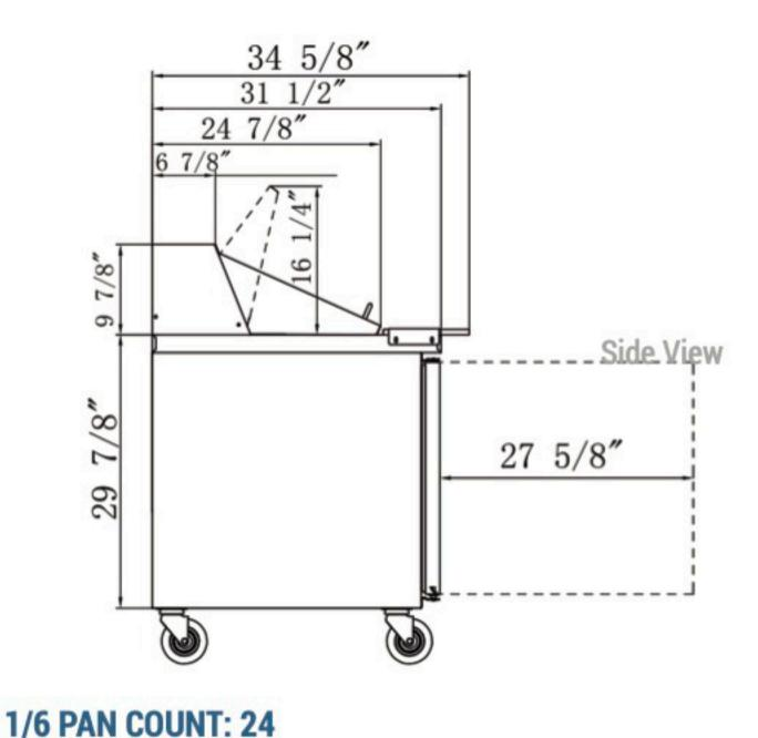
**Cutting Board Size** 60 x 9 Rated Voltage 115V **Rated Frequency** 60Hz **Total Input Power** 280W **Total Current** 2.4A 14.33 cu ft **Total Capacity Climatic Category** 4-5 **Protection Type** Design Pressure High Side **300 PSIG Design Pressure Low Side 150 PSIG Insulation Blowing Gas C-Pentane** Refrigerant R290/3.88 oz
