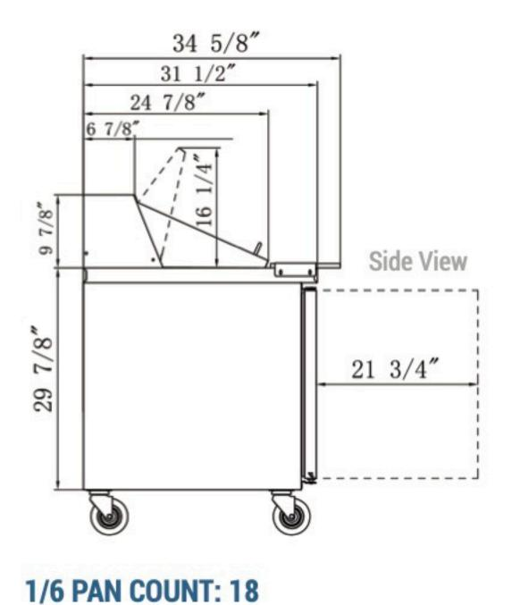
**Cutting Board Size** 48 x 9 Rated Voltage 115V Rated Frequency 60Hz **Total Input Power** 280W **Total Current** 2.4A **Total Capacity** 11.47 cu ft **Climatic Category** 4-5 **Protection Type Design Pressure High Side 300 PSIG Design Pressure Low Side 150 PSIG Insulation Blowing Gas C-Pentane** Refrigerant R290/3.17oz
