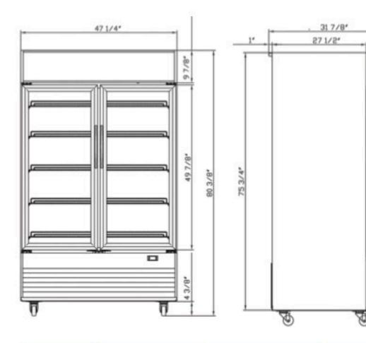
Rated Voltage 1150 Rated Frequency 60Hz 690W **Total Input Power** 8.8A **Total Current Total Capacity** 41.28 cu ft **Climatic Category** 4-5 Protection Type Design Pressure High Side 300 PSIG Design Pressure Low Side 150 PSIG Insulation Blowing Gas C-Pentane Refrigerant R290/2.82 oz
