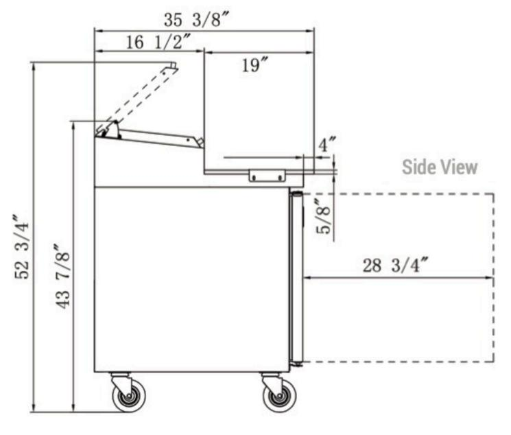
Rated Voltage 115V **Rated Frequency** 60Hz **Total Input Power** 250W 2.2A **Total Current** 9.88 cu ft **Total Capacity Climatic Category** 4-5 **Protection Type** Design Pressure High Side **300 PSIG Design Pressure Low Side 150 PSIG Insulation Blowing Gas C-Pentane** R290/3.7 oz Refrigerant
