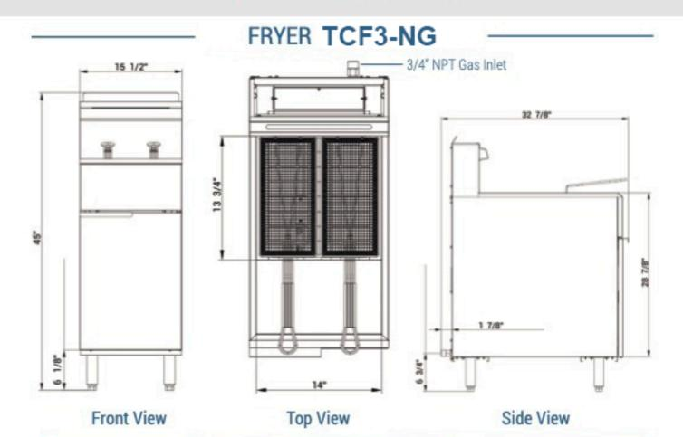
GAS SOURCE NG 14.01x13.98in WORK AREA BURNER 3 count SINGLE BURNER 30000 BTU/H COMBINED 90000 BTU/H **OIL TANK CAPACITY** 40 lbs **GAS PRESSURE** 4 'WC NOZZEL 39# CONTAINER FITMENT 130
