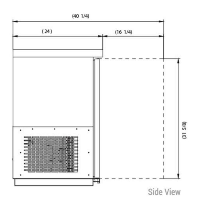
Rated Voltage 115V **Rated Frequency** 60Hz **Total Input Power** 284W 2.66A **Total Current Total Capacity** 11.23 cu ft **Climatic Category** 4-5 **Protection Type** Design Pressure High Side **385 PSIG Design Pressure Low Side 150 PSIG Insulation Blowing Gas C-Pentane** Refrigerant R290/3.17 oz
