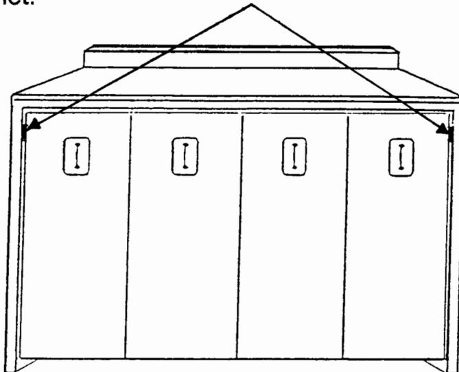
**STEP 15 IS VERY, VERY IMPORTANT!!! YOUR BED MUST BE SECURELY AND CORRECTLY ANCHORED TO THE WALL to assure proper operation and to avoid possible injury.**
