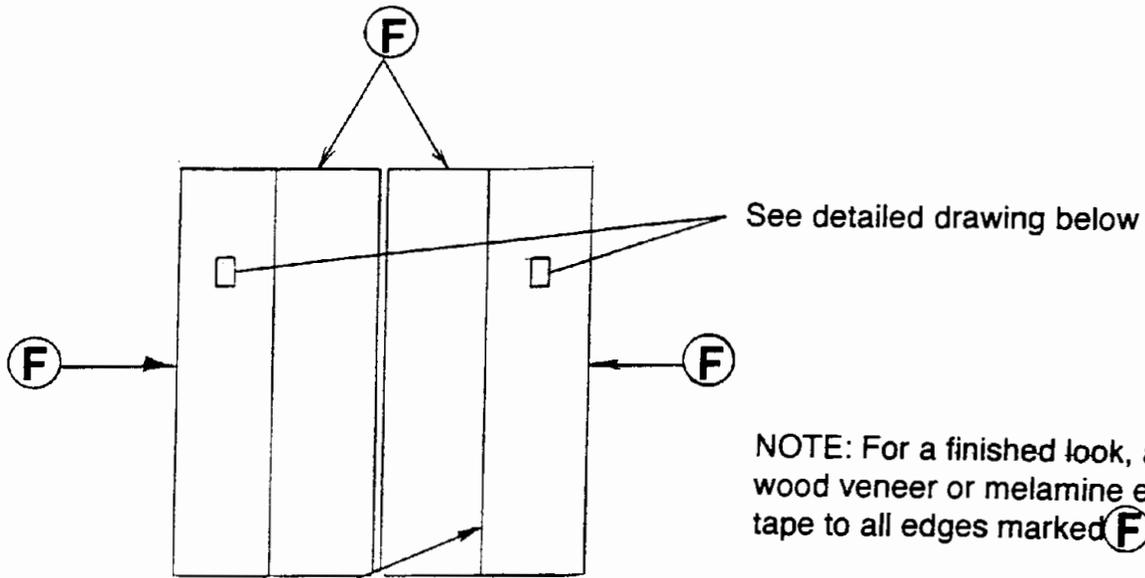
NOTE: For a finished look, apply wood veneer or melamine edge tape to all edges marked **F**
