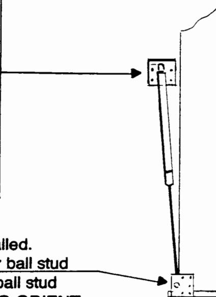
9. At this point, the new piston can be installed. Simply snap the new piston on the lower ball stud located on the bed rail - then the upper ball stud located on the bed vertical. **BE SURE TO ORIENT THE PISTON CORRECTLY** by referring to the label on the piston. ( **MOUNT THIS END UP** )
