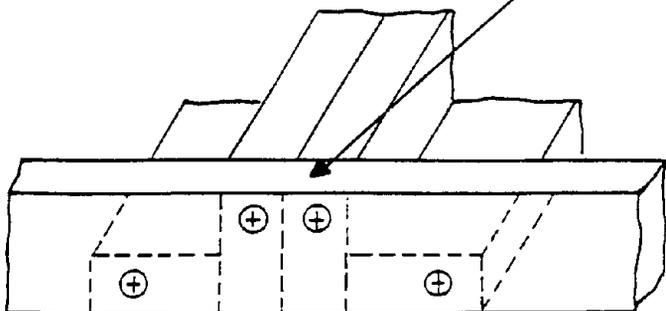
**STEP 3: Mounting the frame struts between the frame sides.**
