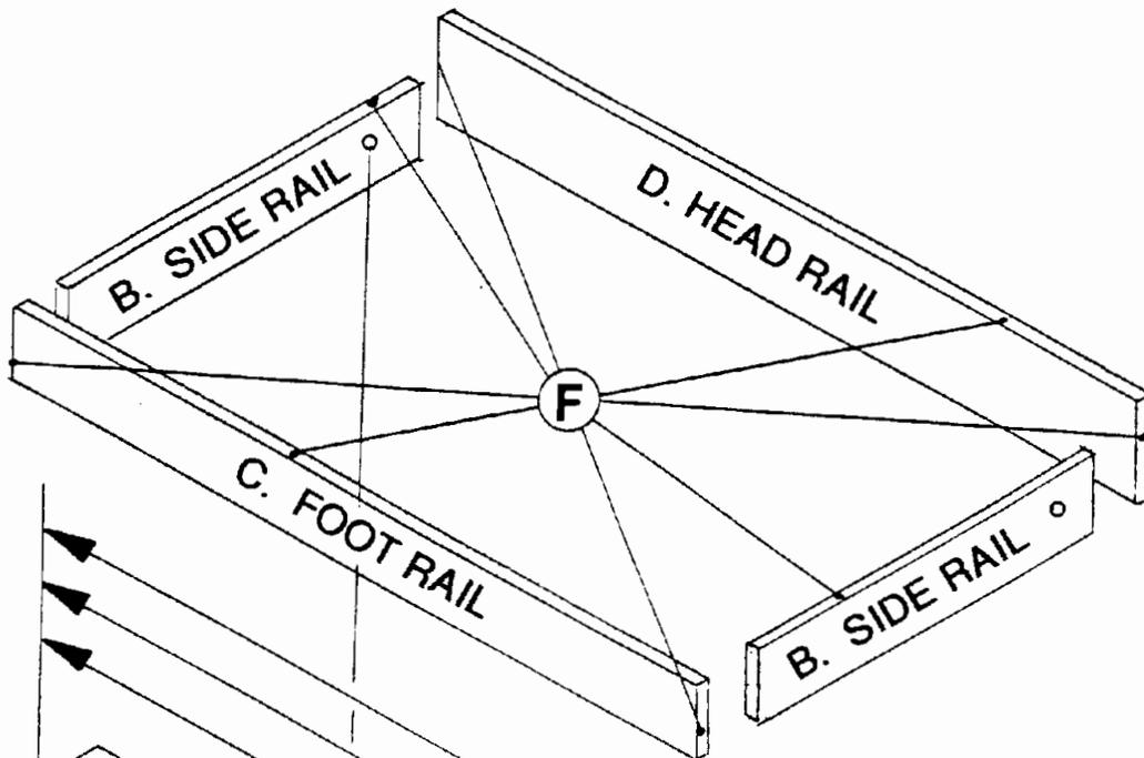
Note: For a finished look, apply wood veneer or melamine edge tape to all edges marked (F)
