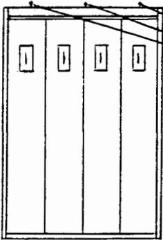
1. With the bed in the upright, closed position with both legs closed and locked, remove the anchor screws from the top of the bed cabinet. Do not remove the anchor screws with the bed in the open position.
