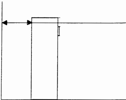
2. Place the bed cabinet 2 to 3 feet away from the wall, allowing enough room to comfortably work behind the bed cabinet.
