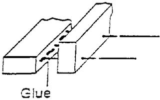
Run a bead of wood glue along inside edge. Making sure ends are flush drill pilot holes approximately 8" apart and nail with 1 1/2" finish nails, or you can use #8 1 1/2" screws.
