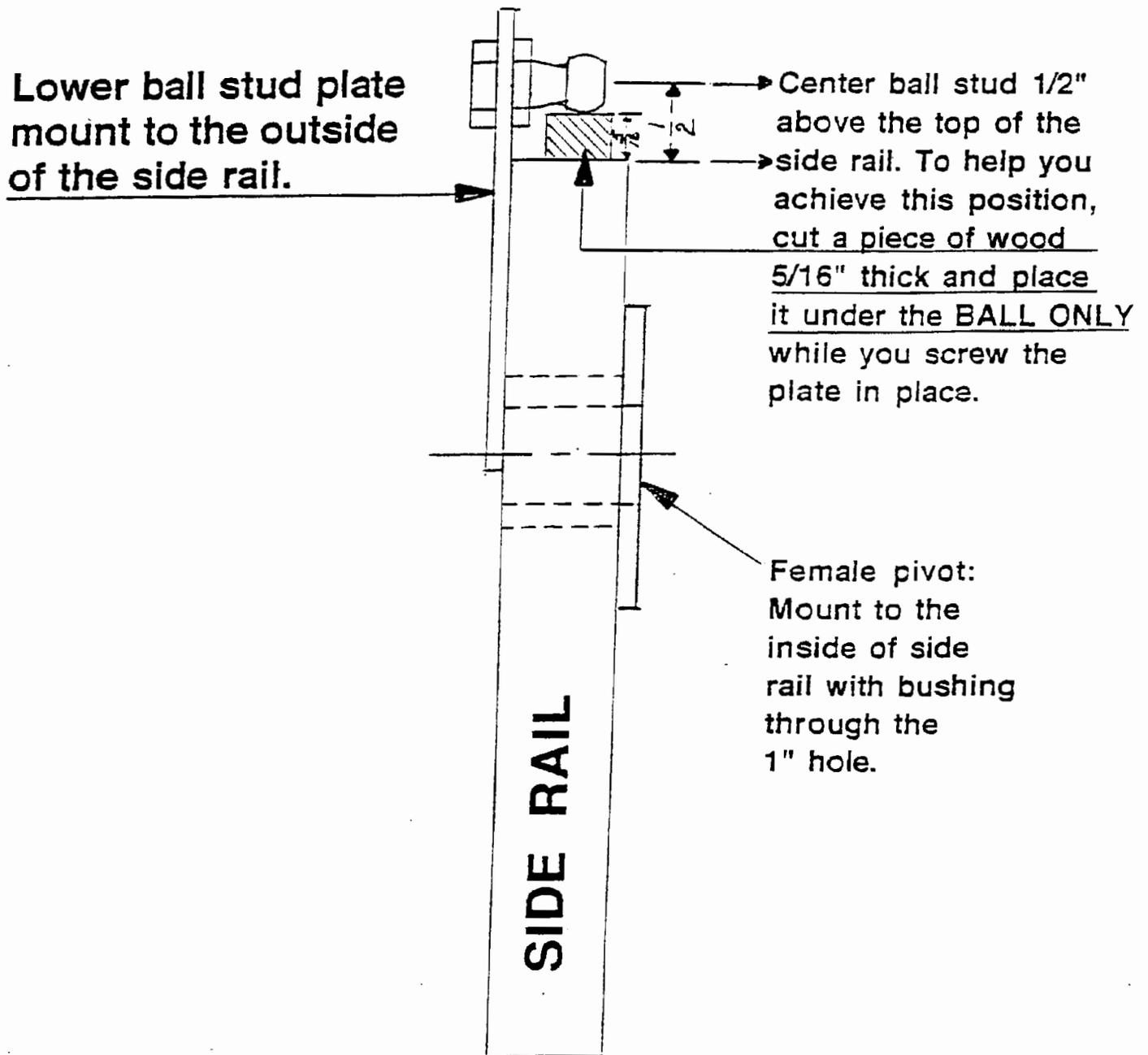
STEP 4: Mounting the lower ball stud plate to the outside of the side rail PARTS B
