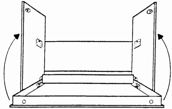
**NOTE:** To prevent damage to the legs be sure they are in the closed position when rotating the bed into the upright position.
