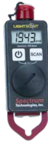
3415A LightScout® Quantum PAR/DLI Light Meter
