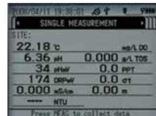
Water quality monitor displays 11 parameters simultaneously
