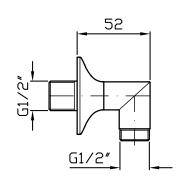
The Bellagio wall elbow has a 1/2" male water inlet connection. Crafted from solid brass.
