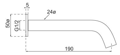
Note: All dimensions are in millimetres and are subject to normal manufacturing variations. Always use the physical product measurements for cut-outs and rough-ins as the technical details shown may differ from the actual product. Use acetic cured silicone sealant. Do not use epoxy type adhesives. Clean with damp cloth. Do not use abrasive cleaners, liquids or pastes.
