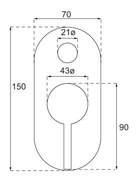
Note: All dimensions are in millimetres and are subject to normal manufacturing variations. Always use the physical product measurements for cut-outs and rough-ins as the technical details shown may differ from the actual product. Use acetic cured silicone sealant. Do not use epoxy type adhesives. Clean with damp cloth. Do not use abrasive cleaners, liquids or pastes.
