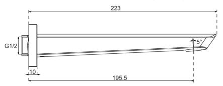
Note: All dimensions are in millimetres and are subject to normal manufacturing variations. Always use the physical product measurements for cut-outs and rough-ins as the technical details shown may differ from the actual product. Use acetic cured silicone sealant. Do not use epoxy type adhesives. Clean with damp cloth. Do not use abrasive cleaners, liquids or pastes.
