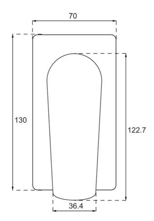
Note: All dimensions are in millimetres and are subject to normal manufacturing variations. Always use the physical product measurements for cut-outs and rough-ins as the technical details shown may differ from the actual product. Use acetic cured silicone sealant. Do not use epoxy type adhesives. Clean with damp cloth. Do not use abrasive cleaners, liquids or pastes.
