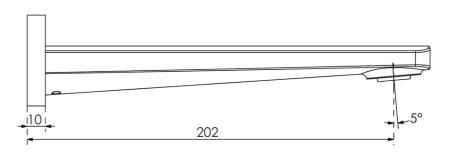
Note: All dimensions are in millimetres and are subject to normal manufacturing variations. Always use the physical product measurements for cut-outs and rough-ins as the technical details shown may differ from the actual product. Use acetic cured silicone sealant. Do not use epoxy type adhesives. Clean with damp cloth. Do not use abrasive cleaners, liquids or pastes.
