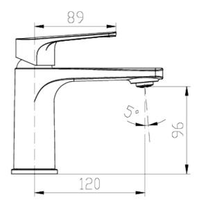
Note: All dimensions are in millimetres and are subject to normal manufacturing variations. Always use the physical product measurements for cut-outs and rough-ins as the technical details shown may differ from the actual product. Use acetic cured silicone sealant. Do not use epoxy type adhesives. Clean with damp cloth. Do not use abrasive cleaners, liquids or pastes.
