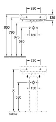
Note: All dimensions are in millimetres and are subject to normal manufacturing variations. Always use the physical product measurements for cut-outs and rough-ins as the technical details shown may differ from the actual product. Use acetic cured silicone sealant. Do not use epoxy type adhesives. Clean with damp cloth. Do not use abrasive cleaners, liquids or pastes.
