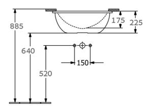
Note: All dimensions are in millimetres and are subject to normal manufacturing variations. Always use the physical product measurements for cut-outs and rough-ins as the technical details shown may differ from the actual product. Use acetic cured silicone sealant. Do not use epoxy type adhesives. Clean with damp cloth. Do not use abrasive cleaners, liquids or pastes.
