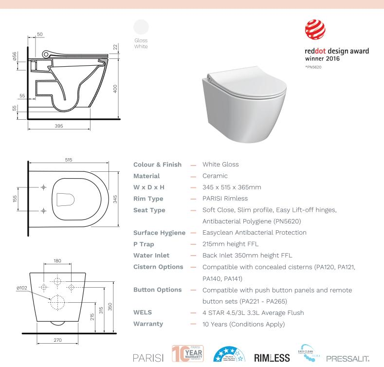
Note: Dimensions are in millimetres and nominal. They can vary according to material and manufacturing tolerances. Exact dimensions should be determined by measuring actual product. PARISI reserves the right to vary specifications without notice. April 2020
