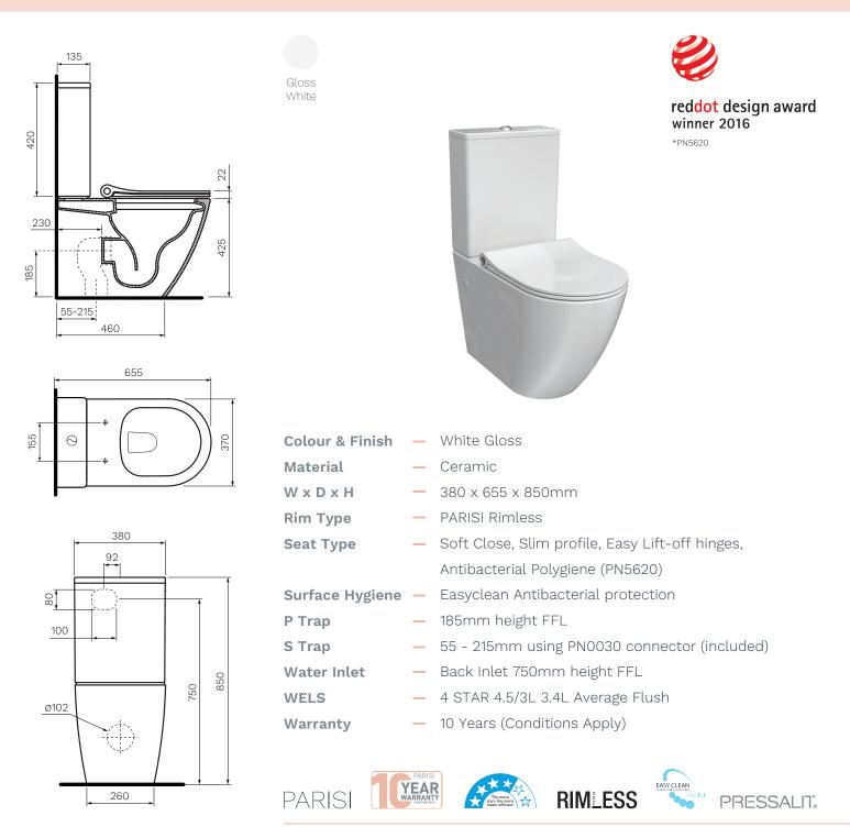
Note: Dimensions are in millimetres and nominal. They can vary according to material and manufacturing tolerances. Exact dimensions should be determined by measuring actual product. PARISI reserves the right to vary specifications without notice. April 2020
