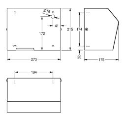
RODAN touch free electronic warm air hand dryer for wall mounting, stainless steel, surface satin finished, front material thickness is 1.2 mm, infrared sensor activity for non-touch operation, sensor range adjustable from 10 to 30 cm, automatic power shut-off after 60 s, cable and plug not included.
