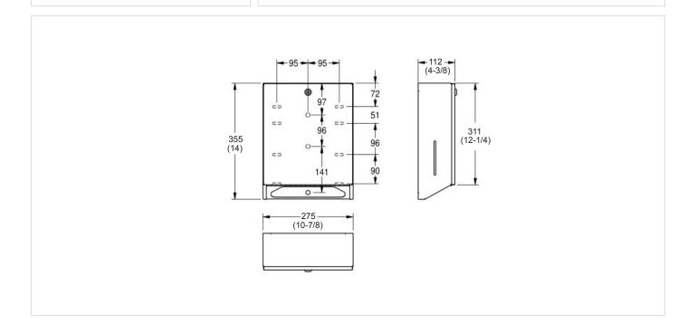
Franke Commercial 'RODAN' #RODX600 Paper Towel Dispenser, 14" H x 10-7/8" W x 4-3/8" D (355mm x 275mm x 112mm), wall mounted, manufactured from 22 gauge (0.8mm), grade 18-10 type 304 stainless steel with satin surface finish, standard Franke keyed cylinder lock and mounting hardware. Uses 500-800 paper towels depending on paper type and fold. Provide adequate backing in wall for support and comply to local codes for barrier-free requirements.
