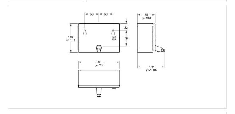
Franke Commercial 'RODAN' #RODX619 Liquid Soap Dispenser, 5-1/2" H x 7-7/8" W x 3-3/8" D (140mm x 200mm x 85mm), wall mounted, manufactured from 22 gauge (0.8mm) grade 18-10 type 304 stainless steel, with satin surface finish, replaceable 34 oz (1L) container suitable for liquid and lotion soaps, standard Franke keyed cylinder lock and mounting hardware. Provide adequate backing in wall for support and comply to local codes for barrier-free requirements.
