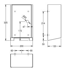
Hand dryer for wall mounting, stainless steel with satin-finish and InoxPlus surface refinement for the reduction of finger marks and better cleaning characteristics (easy to clean), material thickness 1.2 mm, with contactless opto-electronic sensor for touch-free operation, adjustable hot air temperature, sensor range adjustable from 10 to 25 cm, protection from continuous operation with automatic switch-off after 60 seconds, air speed adjustable, cable and plug not included.
