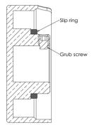
22. Rotate the handle clockwise through approximately 60 degrees until the waveform passes over the small **fastening hole** in the **dress ring**. Insert the Allen key through the hole and tighten the handle in place by fastening the grub screw onto the adaptor. Make sure the handle is pushed up against the wall when tightening.
