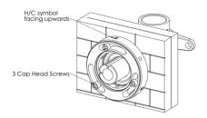
19. To ensure that the dress ring is perfectly concentric to the valve, we have supplied a round plastic **concentricity spacer**. Slide this over the **splined adaptor** and locate it into the **dress ring**, then lock up the 3 **cap head screws**.
