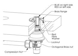
9. Check that the Copper Tee-piece is properly inserted into the spout assembly (the O-rings should not be visible), then firmly tighten up the compression nuts on either end of the Copper Tee-piece.
