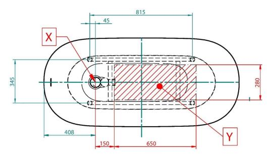
X - Bathtub drain centre Y - Floor waste position Monz Apartment Bath 1400 Floor Waste Position (Model 30809)
