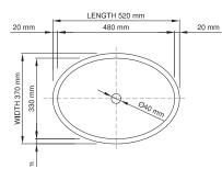
Size (l) x (w) x (h): Top to waste: Overflow: Material: Finish: Mounting: 520mm x 370mm x 110mm 100mm No overflow DADOquartz® Matte / Satin Counter-top / Under-mount
