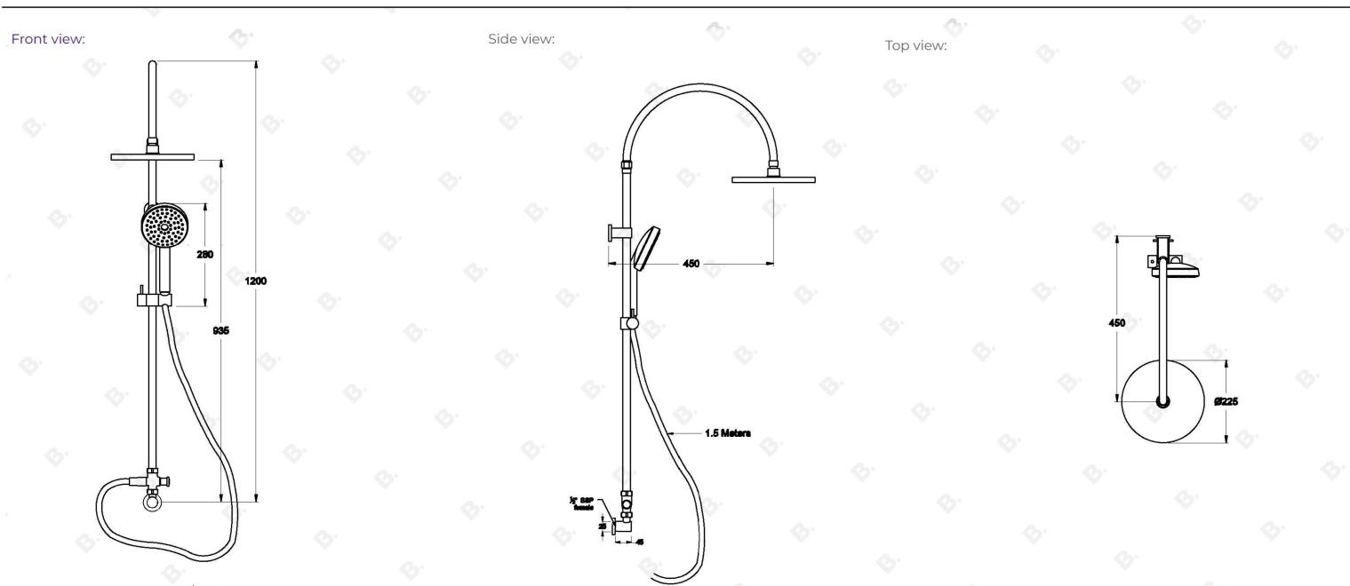
Note: bottom inlet feed requires  $\frac{1}{2}$ " BSP male thread in wall
