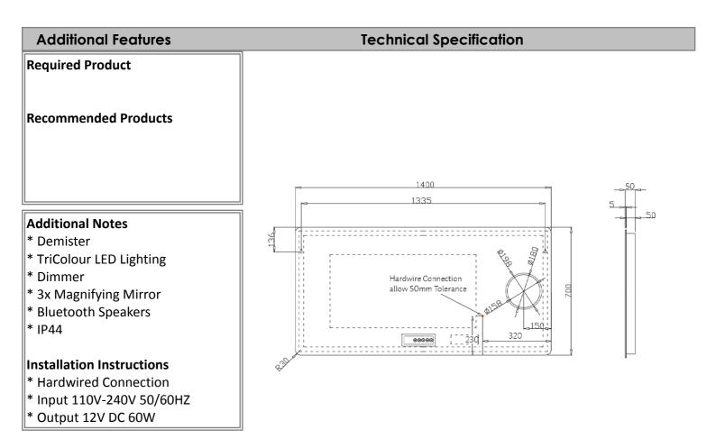
Note: All dimensions are in millimetres and are subject to normal manufacturing variations. Always use the physical product measurements for cut-outs and rough-ins as the technical details shown may differ from the actual product. Use acetic cured silicone sealant. Do not use epoxy type adhesives. Clean with damp cloth. Do not use abrasive cleaners, liquids or pastes.
