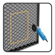
Following steps 1-3 of previous instructions. Using an angle grinder, cut out the opening.
