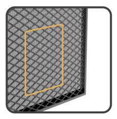
Tape and mark up the measurements needed to cut the opening.
