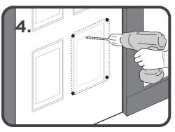
Drill a hole in all four corners with a minimum of 10mm drill bit.
