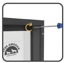
**4.** Push down the strip/bar to clasp the flap in place and secure with screws
