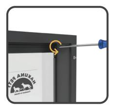
**1.** Remove the screws at the top of the frame securing the flap
