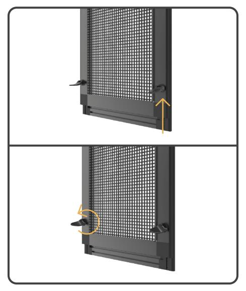
Lift latches and twist to unlock.
