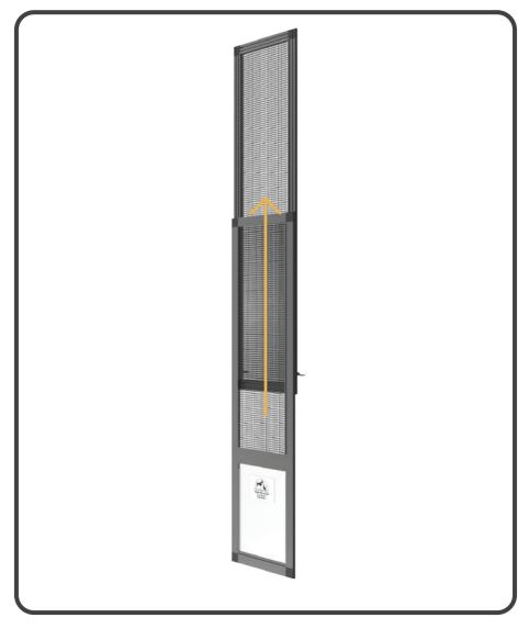
Insert pet door into slidig door track and slide up to extend.
