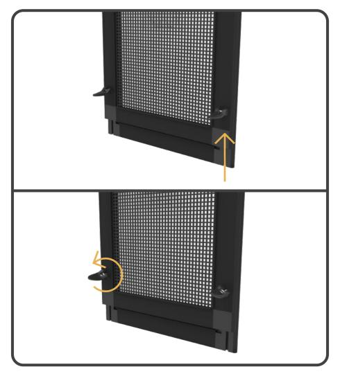
Lift latches and twist to unlock.
