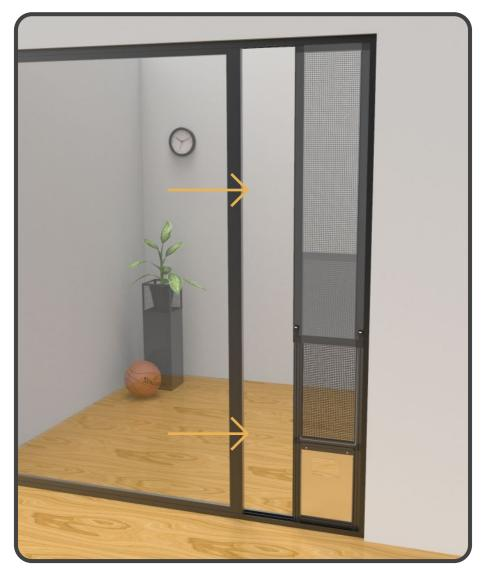
Secure pet door in place by sliding door flush up against pet door frame edge. Note: Ensure sliding door is level, most doors will have adjustment screws to acheive this.
