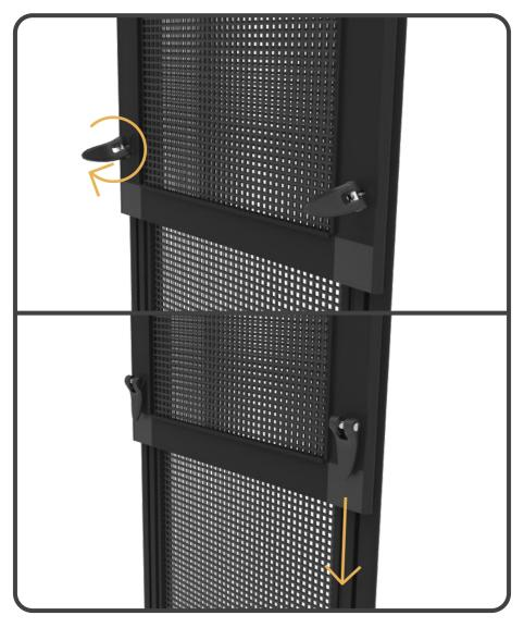
Once extended to fit into sliding door frame, twist and clip down latches to lock. Note: DO NOT over tighten the latches as this will cause damage to the door. Latches are only required to be firm when locking the door in place.
