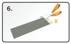
Measure thickness of door/panel and add 10mm (3/8") (x) so tunnel protrudes each side. Cut partition down to correct size.
