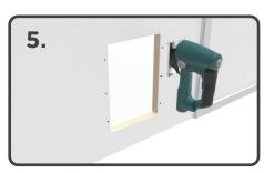
Using a reciprocating jigsaw, cut along marked lines.
