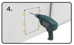
Drill a hole in each of the 4 inside corners with a minimum of 10mm (0.4") drill bit. Then, Drill 6 x 5mm (0.2") pilot holes as circled above.
