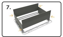
1. Fit all 4 partitions into outer door frame. 2. Duct Tape Corners
