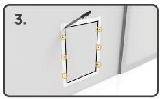
Cut out supplied template, line up height (x) with opening and trace on to door, mark screw holes.
