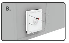
Choose the set of screws that match the thickness of your door frame and screw into door from the inside. WARNING: Over tightening of screws will cause damage.
