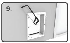
If screws protrude, trim using a hacksaw. Take care when trimming bolts to size as cutting on an angle may cause sharp edges or damage to frame.
